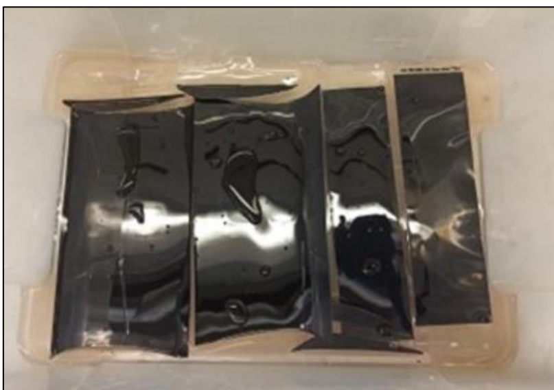
Figure 8: Thermoformed PC sample during the leaching operation
