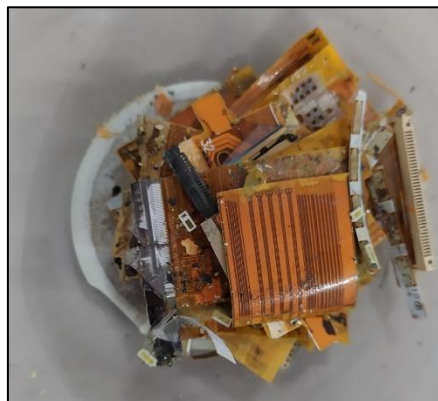
Figure 8: Solid residue of mixture of components after leaching (material from Pollini dashboards)
