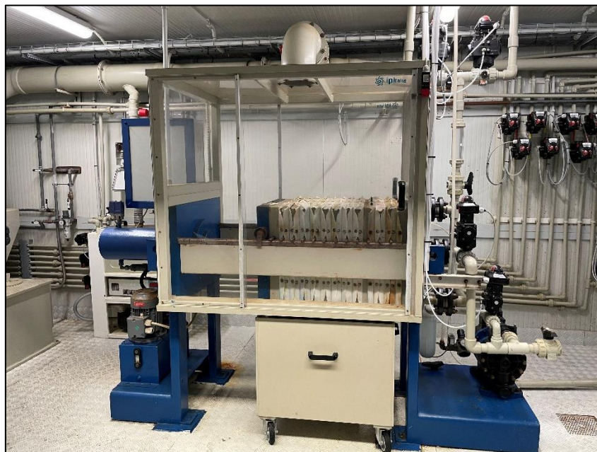
Figure 24: Picture of the plate & frame module in which you can see the polypropylene cart.
