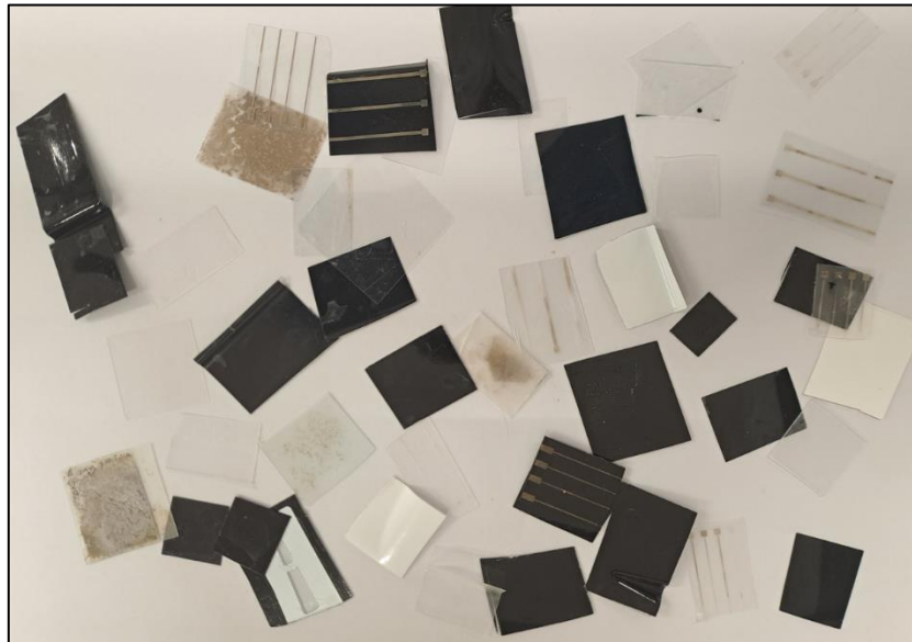
Figure 19: Photographic aspect of a mixture of IME samples after two-steps of leaching
