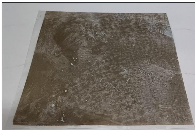
Figure 15: Full silver board IMSE after the hydrometallurgical operation to recover silver.
