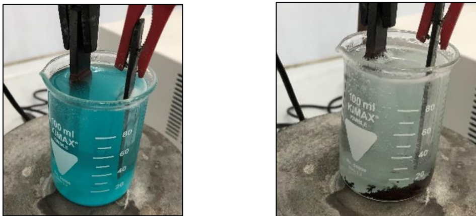
Figure 5: Copper recovery from electrowinning (at the beginning and at the end of the test)
