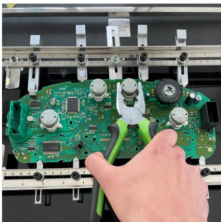
Figure 12 – Disassembly operation of SMD components
