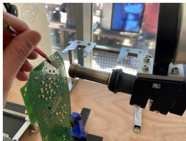
Figure 11 – Disassembly operation of SMD components
