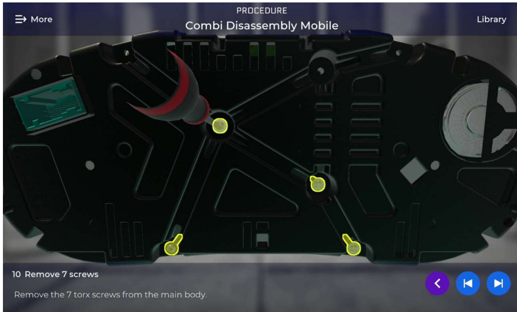
Figure 3.17 - Combimeter disassembly procedure, example step 10
