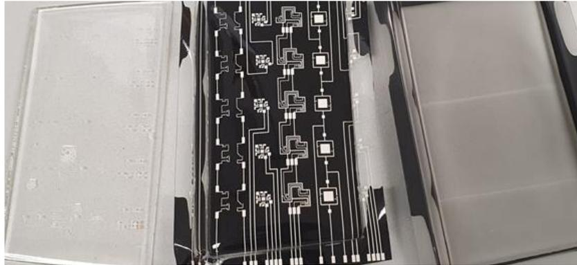
*Figure 24: manual disassembly of the backside of an IME device: a) removal of the epoxy backfill, b) showing the Ag/epoxy interface, c) clean epoxy interface after washing*
