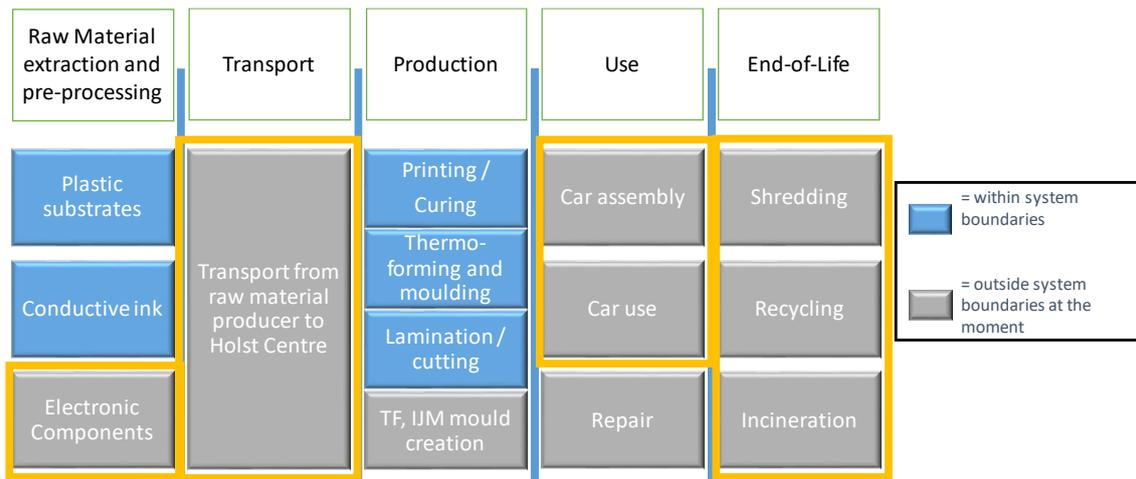
Figure 13: System boundaries for the IME device. Blue boxes represent processes within the system boundaries while grey boxes represent the processes left out of the system boundaries. Orange encircled boxes will be the focus of further study/quantification
