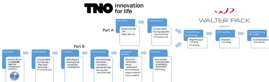
Figure 8: process flow for IME devices created with a 2-foil approach in the EU TREASURE project
