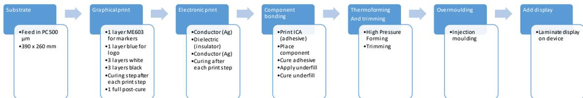
Figure 4: process flow for single-foil IME
