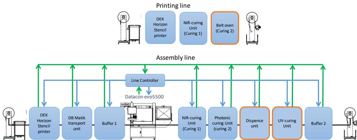
Figure 6: modules added to the roll-to-roll flexible electronics line at Holst Centre in the course of 2022 are indicated by orange lines
