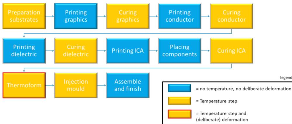
Figure 14: production process of the IME touch panel
