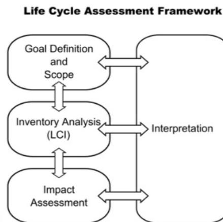
Figure 12: Standard procedure in a Life Cycle Assessment
