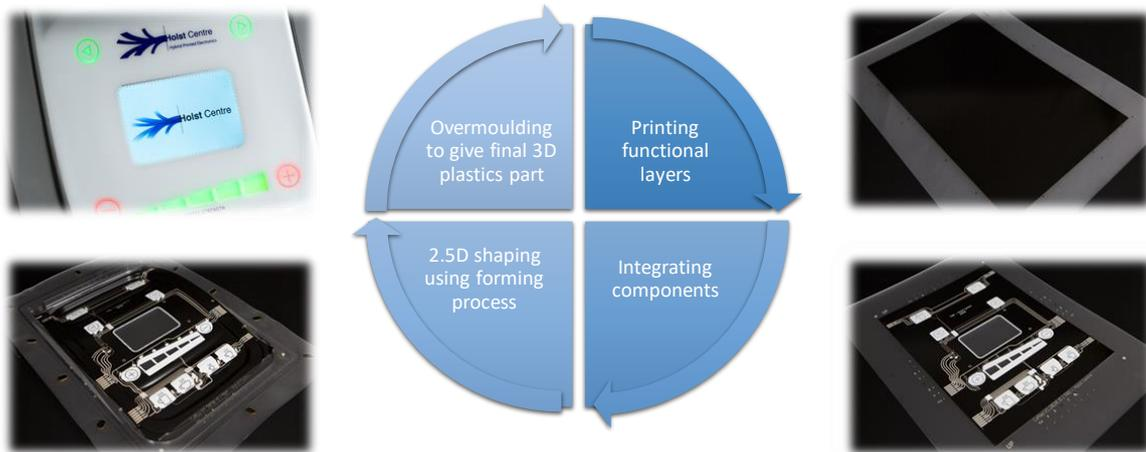
Figure 2: rough process flow for single-foil IME-based coffee machine interface panel
