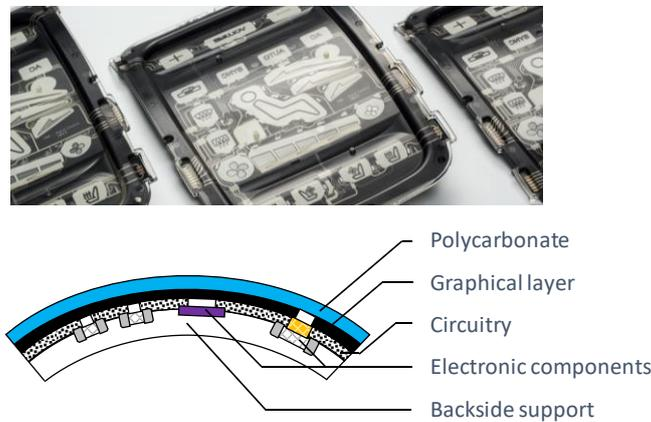
Figure 3: layer stacking for single-foil IME
