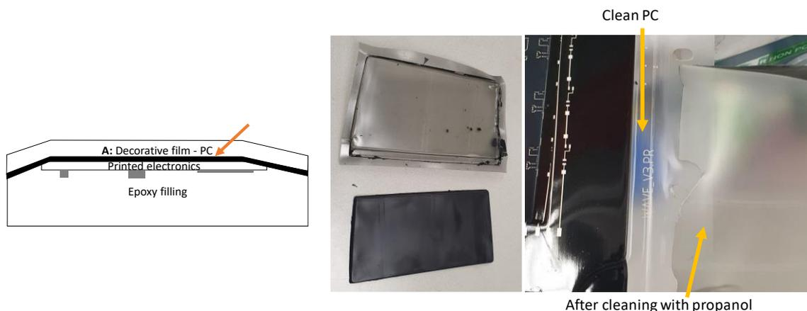
Figure 21: photonic debonding of an IME device
