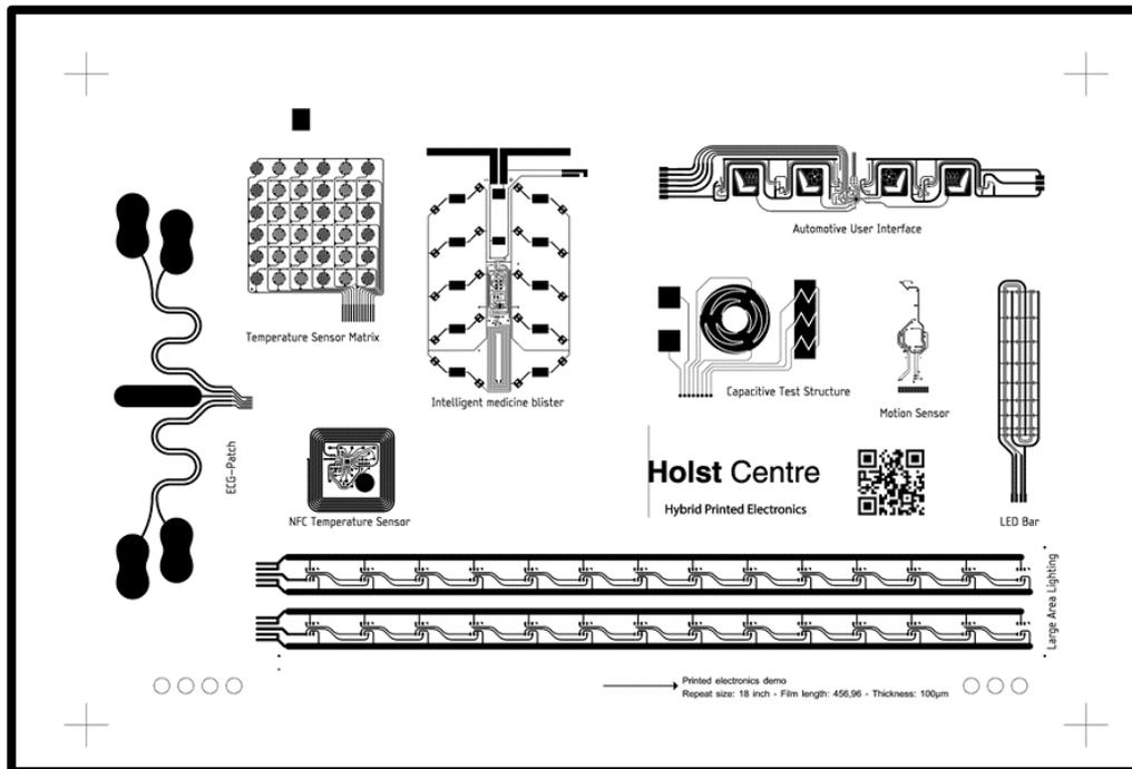
Figure 9: layout of the printed electronics in the R2R test run
