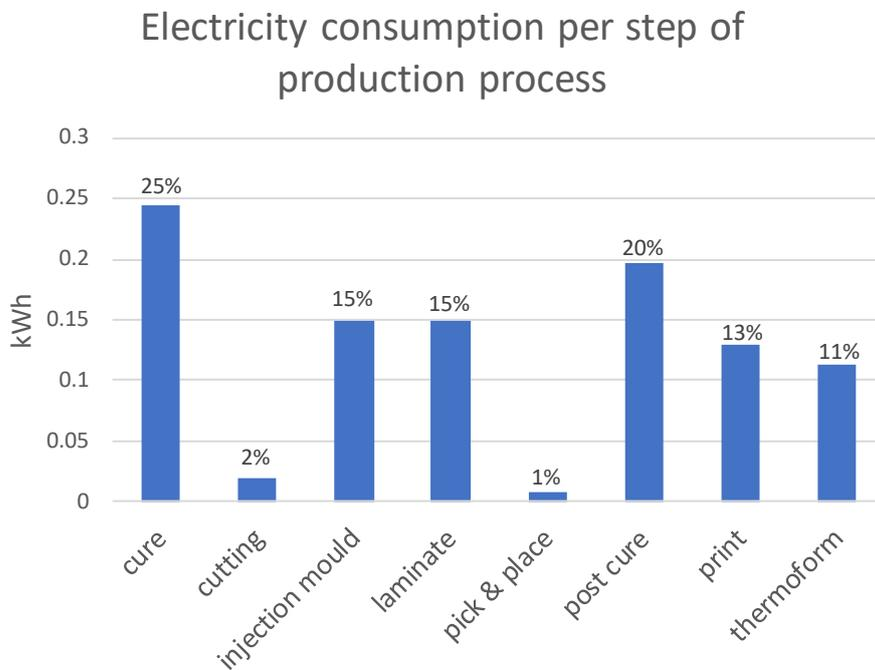
Figure 19: Electricity consumption in kWh per product and per process for the IME panel
