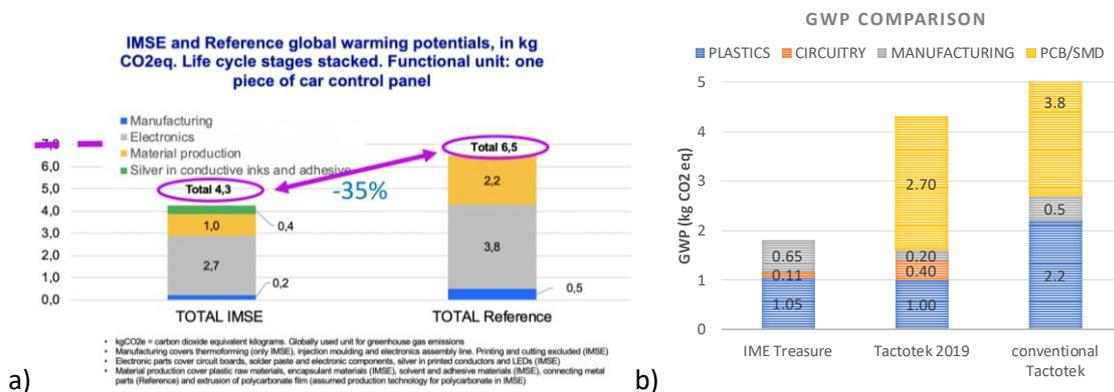
Figure 20: a) LCA by VTT at the request of Tactotek<sup>6</sup>, b) comparison of the LCA in this report and the Tactotek LCA for panels based on IME and conventional electronics<sup>8,8</sup>
