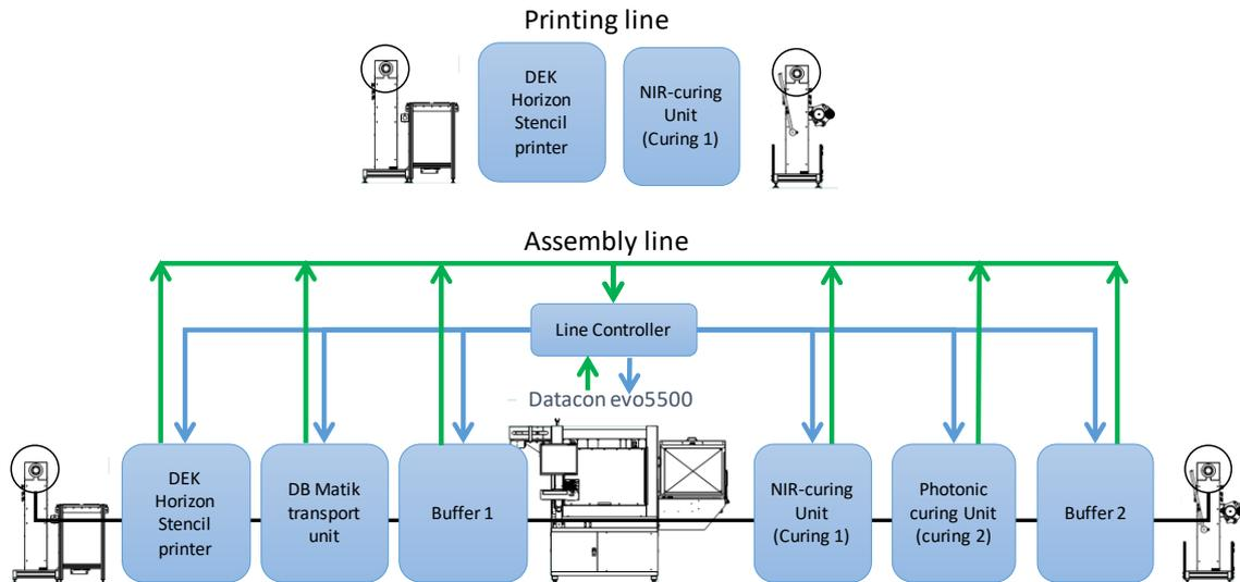
Figure 5: Roll-to-roll flexible electronics line at Holst Centre at the end of the InScope project
