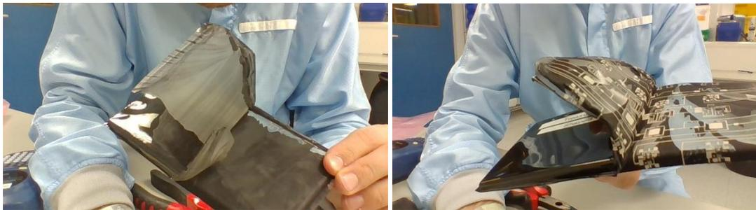
Figure 22: manual disassembly of an IME device with different results: a) rupture at the interface of PC and graphic ink, b) rupture at various interfaces
