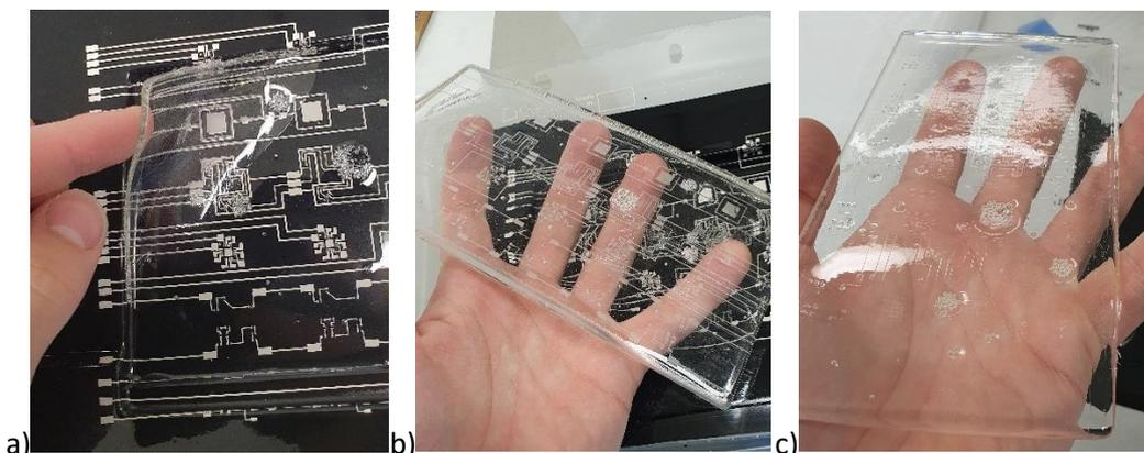
*Figure 23: manual disassembly of the backside of an IME device: a) removal of the epoxy backfill, b) showing the Ag/epoxy interface, c) clean epoxy interface after washing*
