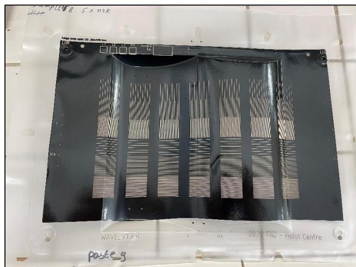
Figure 3. In-mold electronics: thermoformed sample B.
