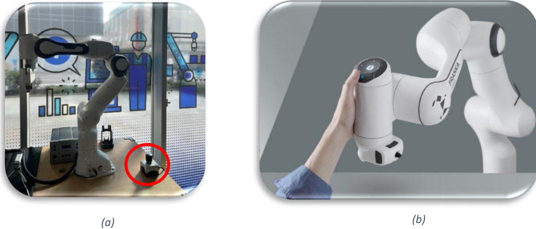
Figure 5 – Manual Guidance for the Franka Emika Panda Cobot
