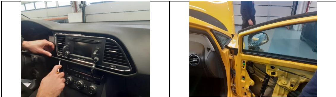
Figure 10: Disassembly Level 1 for infotainment (left) and exterior mirror (right). Source: D3.2.
