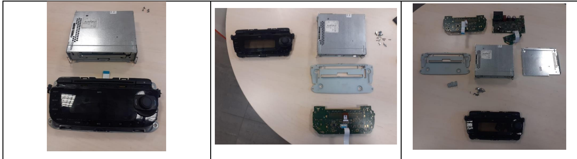
Figure 20: Infotainment level 2 disassembly process – SEAT Ibiza model IV
