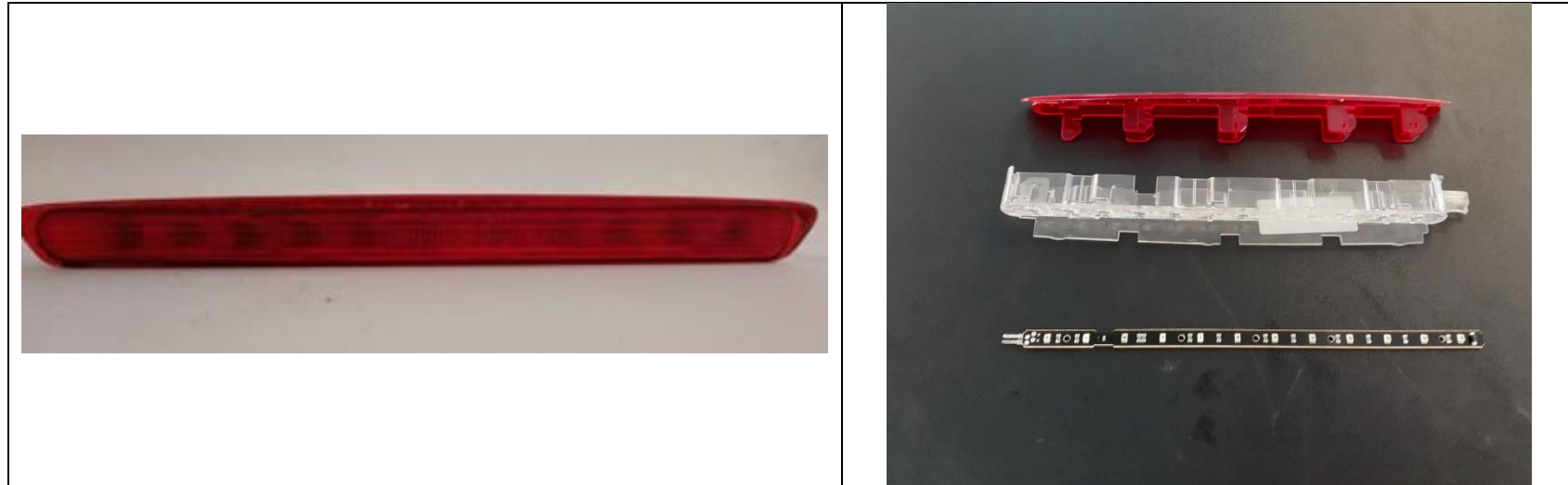
Figure 35: Additional brake lighting level 2 disassembly process – SEAT Ibiza model IV
