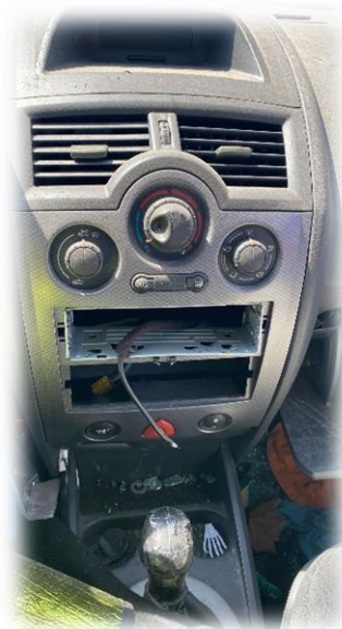
A vehicle that arrived at an ELV authorised centre without the infotainment
