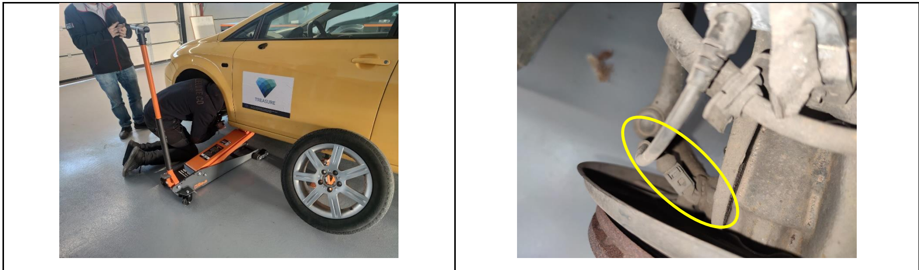
Figure 37: Speed sensor level 1 disassembly process – SEAT Leon model II
