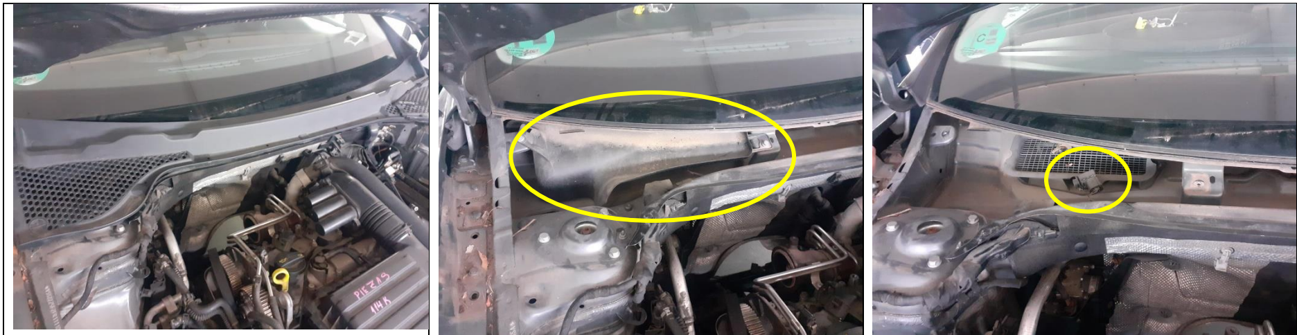
Figure 46: Air quality sensor level 1 disassembly process – SEAT Leon model III
