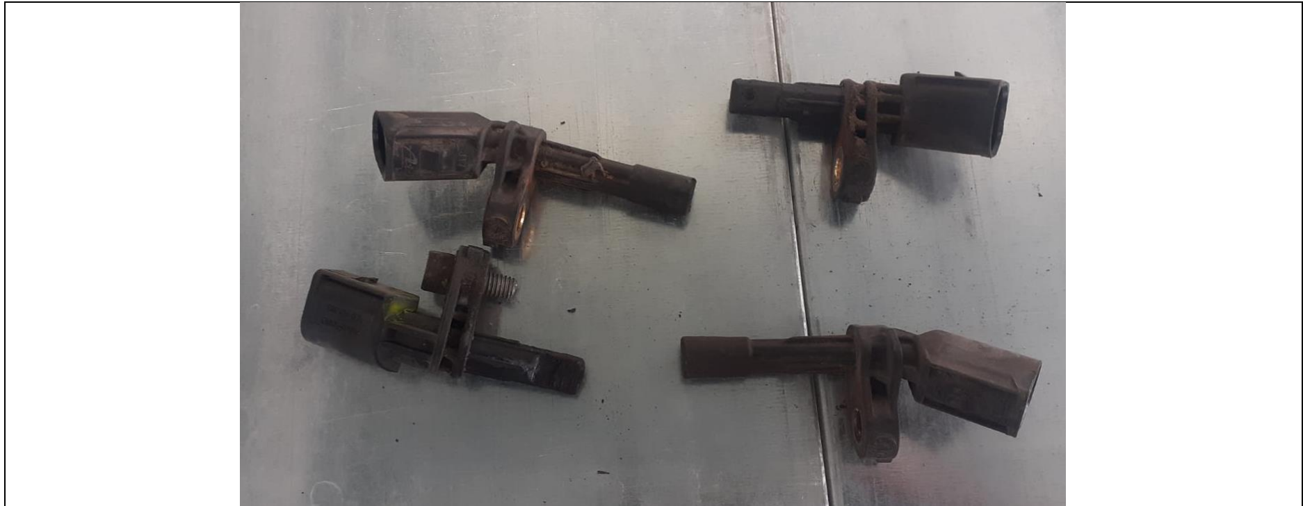
Figure 38: Speed sensor level 2-3 disassembly process – SEAT Leon model II
