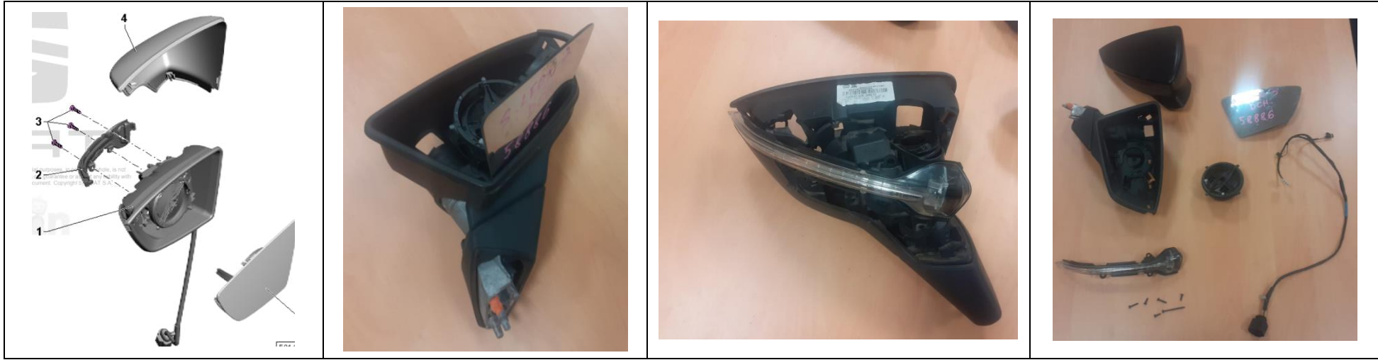
Figure 26: Exterior mirror level 2 disassembly process – SEAT Leon model III
