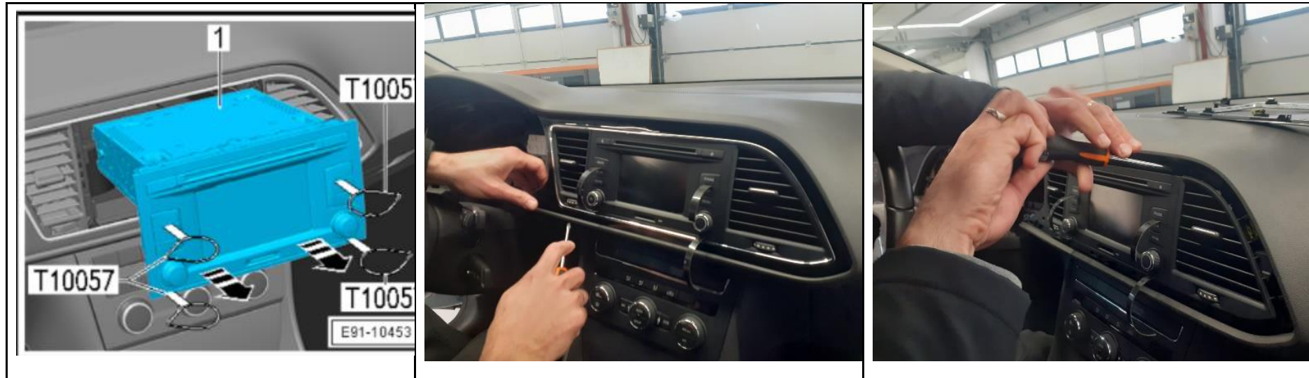
Figure 16: Infotainment level 1 disassembly process – SEAT Leon model III
