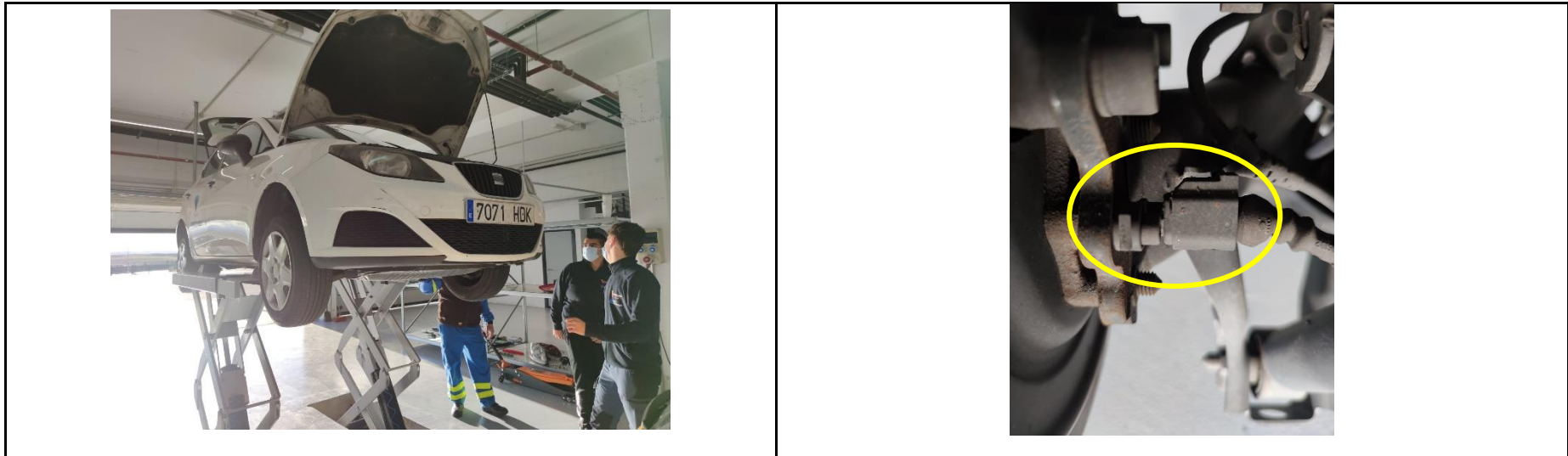
Figure 41: Speed sensor level 1 disassembly process – SEAT Ibiza model IV
