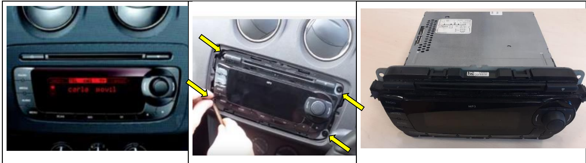
Figure 19: Infotainment level 1 disassembly process – SEAT Ibiza model IV
