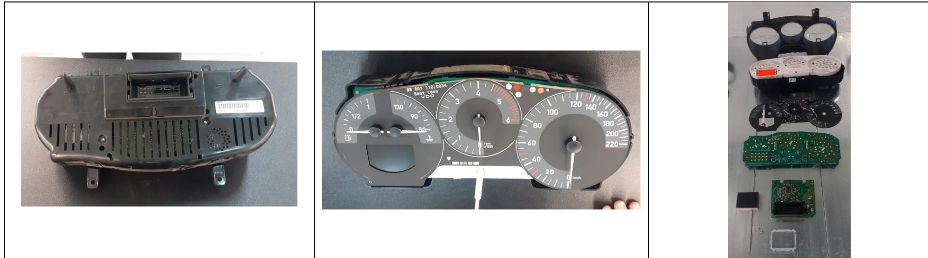
Figure 5: Combi Instrument level 2 disassembly process – SEAT Leon model II
