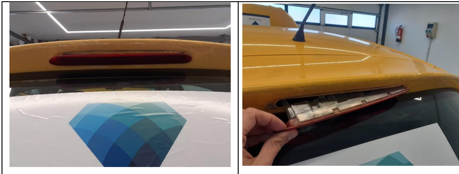
Figure 28: Additional brake lighting level 1 disassembly process – SEAT Leon model II
