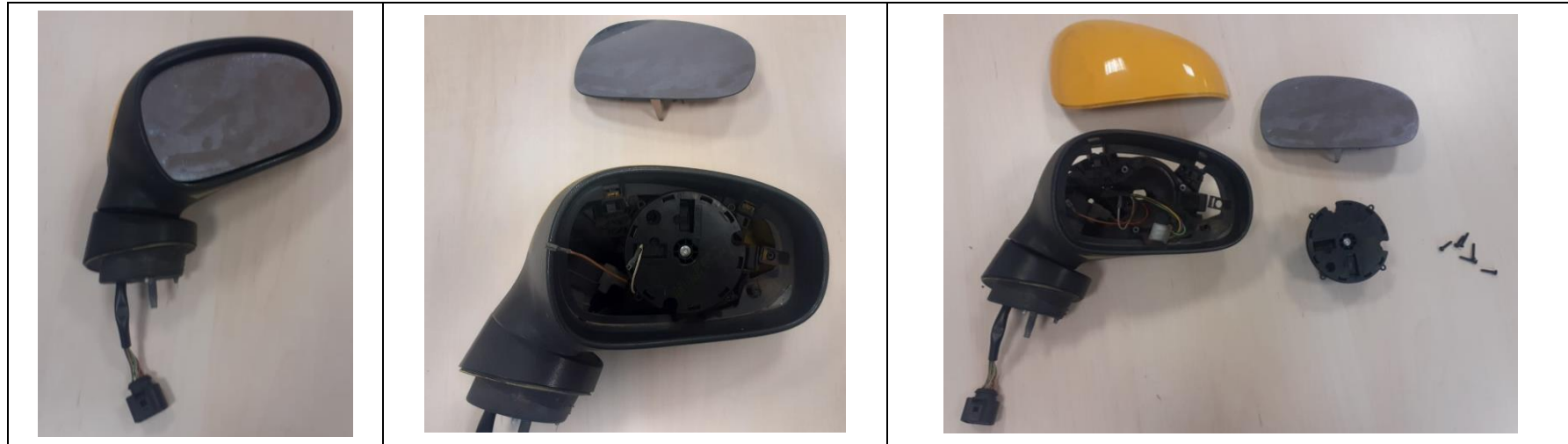
Figure 23: Exterior mirror level 2 disassembly process – SEAT Leon model II
