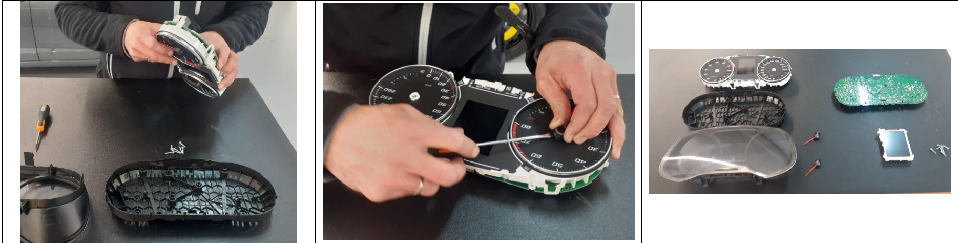
Figure 8: Combi Instrument level 2 disassembly process – SEAT Leon model III
