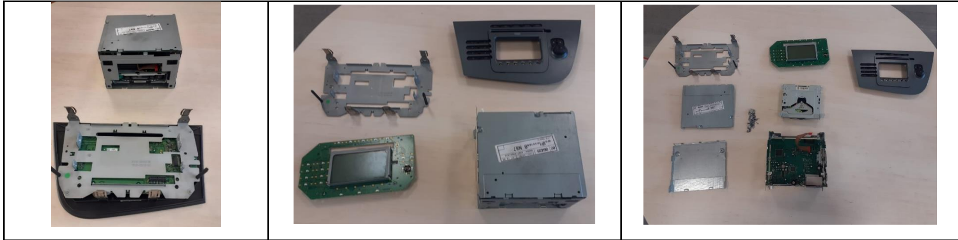
Figure 14: Infotainment level 2 disassembly process – SEAT Leon model II
