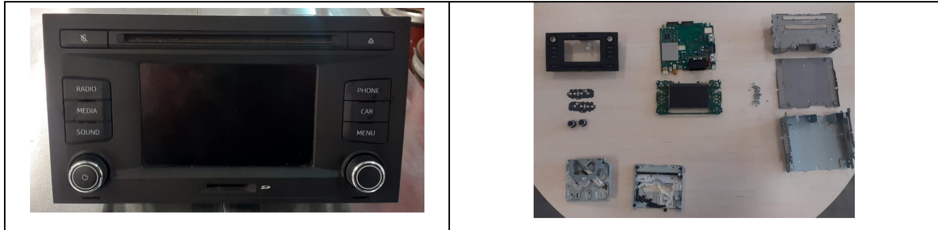
Figure 17: Infotainment level 2 disassembly process – SEAT Leon model III
