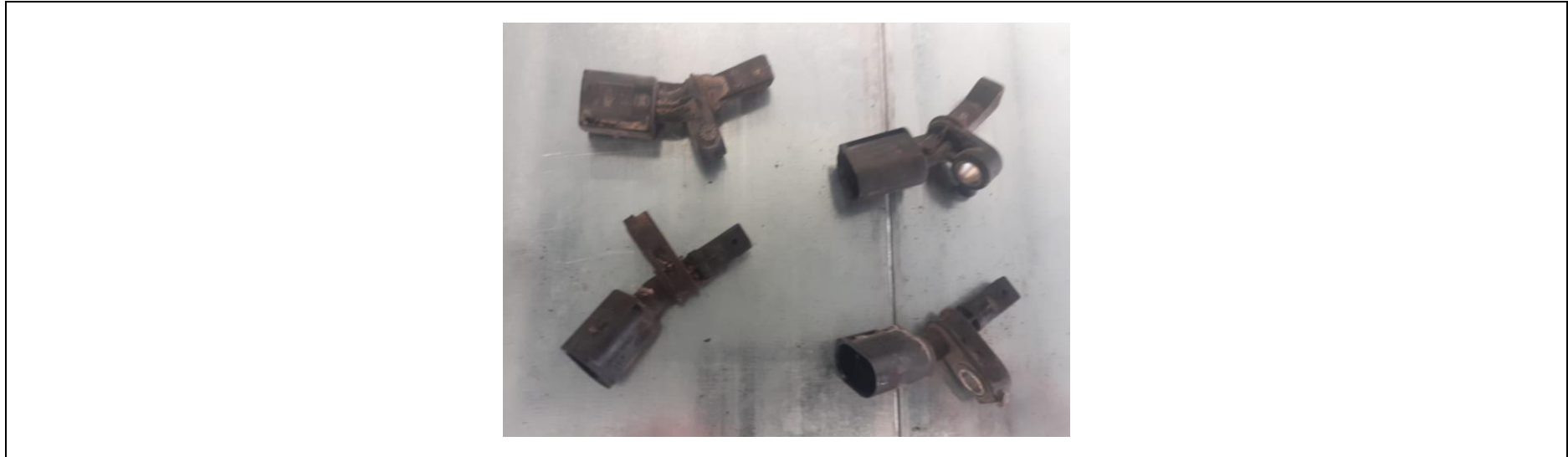
Figure 42: Speed sensor level 2-3 disassembly process – SEAT Ibiza model IV
