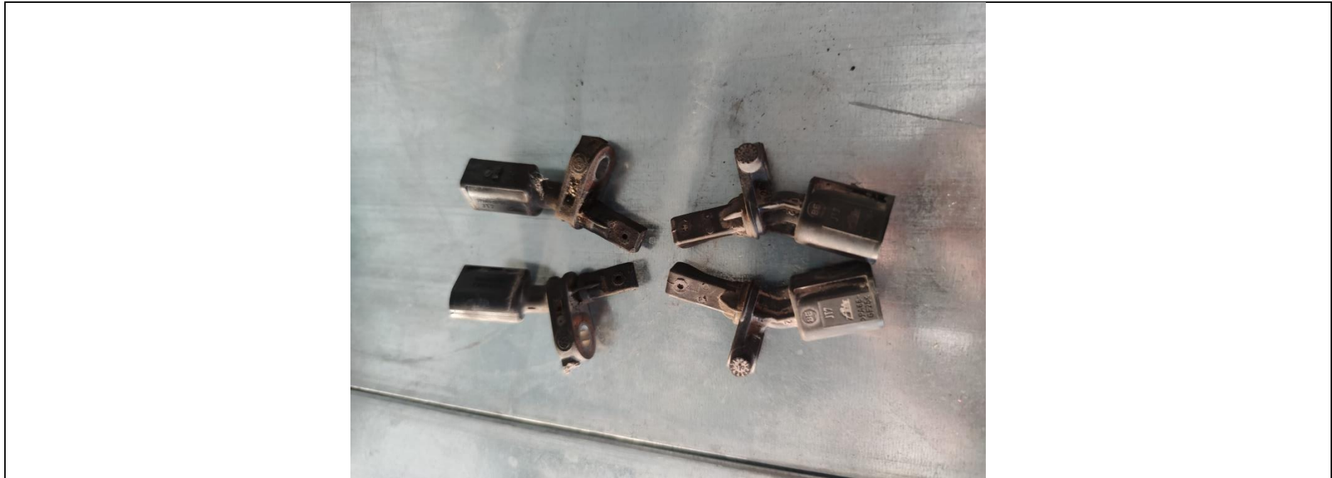
Figure 40: Speed sensor level 2-3 disassembly process – SEAT Leon model III
