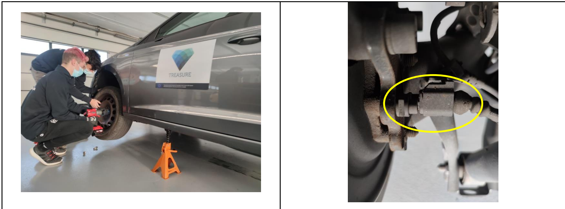
Figure 39: Speed sensor level 1 disassembly process – SEAT Leon model III
