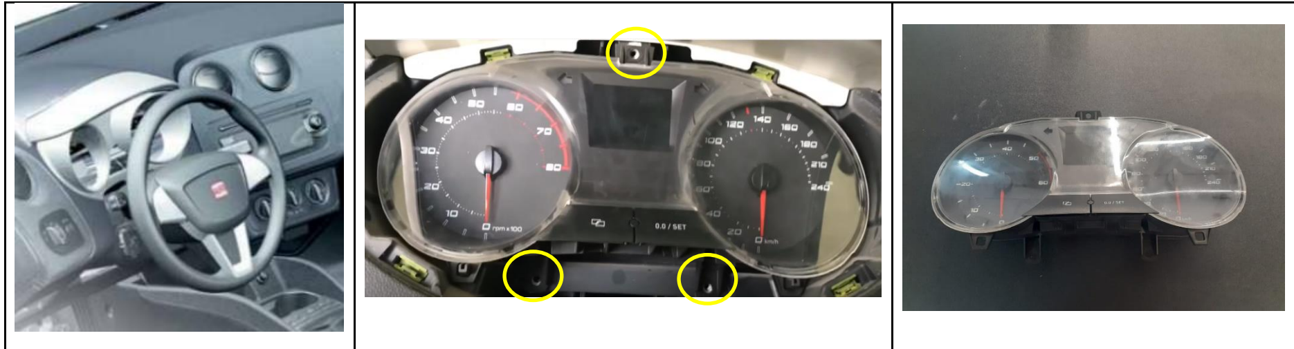
Figure 10: Combi Instrument level 1 disassembly process – SEAT Ibiza model IV
